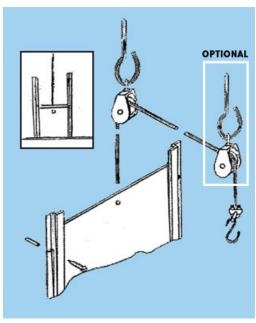
Place panel against wall as a template. Install each channel so the panel slides in its grooved track.
