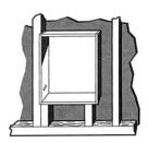
Example of tunnel in frame wall
